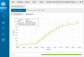
PAS Software adopts a unique intake control method, the pressure in adsorption and desorption process is optimally set in six-stage; this flexible design is helpful for improving test efficiency.
