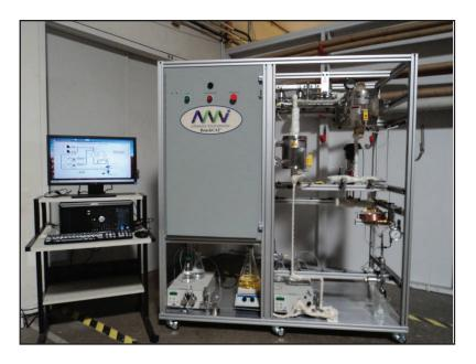
Figure 4. BenchCAT reactor for supercritical trans-esterification of lipids.
