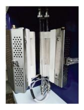
Fully independent detection system can detect three samples simultaneously without interacting with the results of different detection channels. The three detection channels share the same heating furnace and perform excellently when the test requirements are high.
