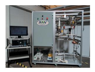
These Catalytic Test Units (CTUs) can be used for many specialty chemical processes, fine chemical and pharmaceutical chemistries, such as: hydrogenation, amination and dehydrochlorination. When used with Applied Catalysts activated carbon monolith catalysts (ACMC®), in addition to process intensification (high productivity), the advantages include: higher selectivity, better thermal management, and low pressure drop/low attrition.
