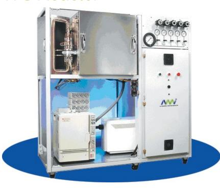
reactor tubes using a set of matched capillaries. A single closure is required to seal all eight reactors. The reactor effluents are routed through heated lines to a condenser and a multiposition selector valve. Analysis of the products is accomplished by gas chromatography. The unit was designed to hold up to 10 mL of catalyst in each reactor and operate at 650 C and 800 psig.
