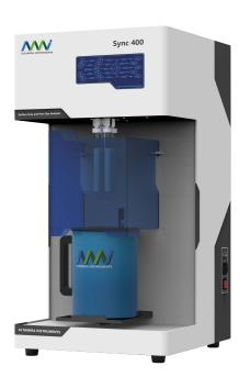
**Altamira** With the AMI-sync series, offers a high-throughput instrument with up to four measuring stations and a separate po measuring cell for measurement of simultaneous saturation vapor pressure. The AMI-sync can be equipped as a 1-, 2- or 4station instrument. This high-throughput instrument offers versatility for any laboratory.
