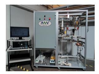
These Catalytic Test Units (CTUs) can be used for many specialty chemical processes, fine chemical and pharmaceutical chemistries, such as: hydrogenation, amination and dehydrochlorination. When used with Applied Catalysts activated carbon monolith catalysts (ACMC<sup>®</sup>), in addition to process intensification (high productivity), the advantages include: higher selectivity, better thermal management, and low pressure drop/low attrition.
