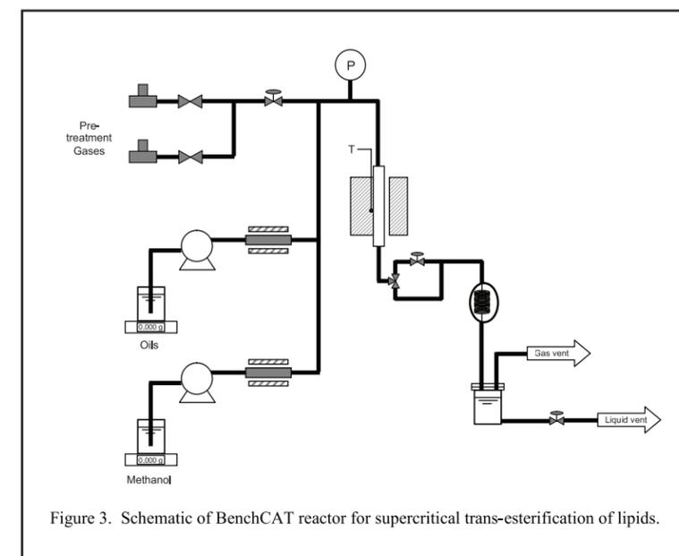
Figure 3. Schematic of BenchCAT reactor for supercritical trans-esterification of lipids.
