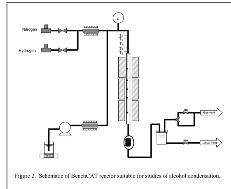
Figure 2. Schematic of BenchCAT reactor suitable for studies of alcohol condensation.
