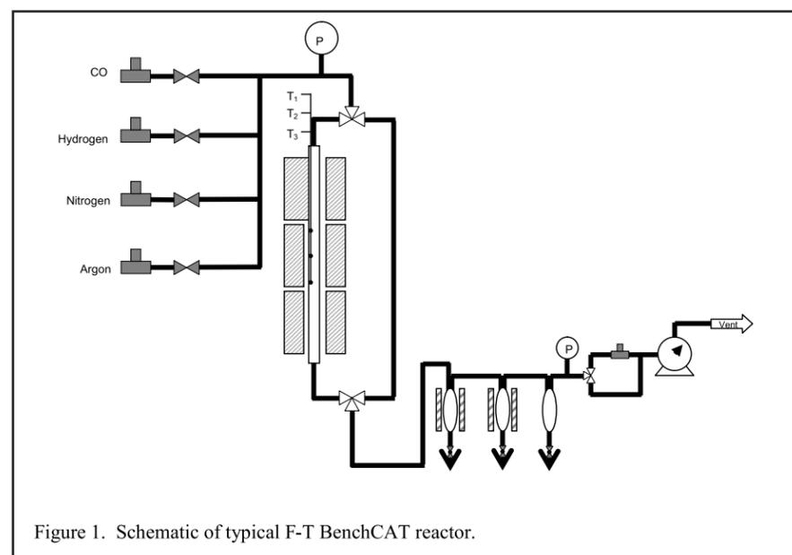
Figure 1. Schematic of typical F-T BenchCAT reactor.
