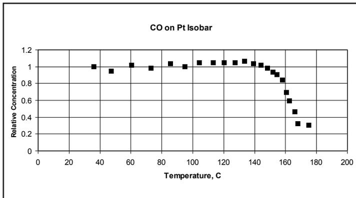
Figure 6. Isobar of CO adsorbed on 1% Pt/Al<sub>2</sub>O<sub>3</sub>.
