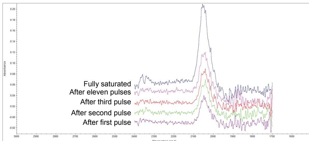
Figure 8. Pulse chemisorption of CO on Pt by FTIR.
