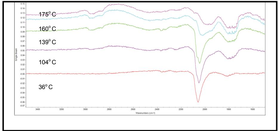
Figure 5. CO signal as a function of temperature.
