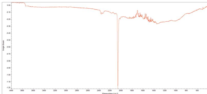
Figure 4. IR spectrum of CO adsorbed on a 1% Pt/Al<sub>2</sub>O<sub>3</sub> catalyst.
