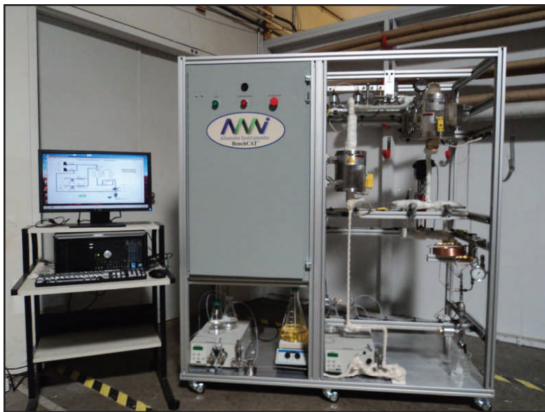
Figure 4. BenchCAT reactor for supercritical trans-esterification of lipids.
