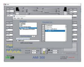
Experimental program setup interface Flexible selection or editing of TPD, TPO, TPR, TPRS, pulse calibration, etc., can set up to 99 programs to achieve full automation of adsorption, desorption, and chemical reactions. The complete experiment setup can be completed within a few minutes.
