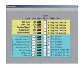
Security protection program settings interface The software has an alarm program, which can realize various safety protection mechanism settings. In manual mode, you can switch any valve by simply clicking on the icon with the mouse. Gas flow rate and temperature values can be entered from the page.
