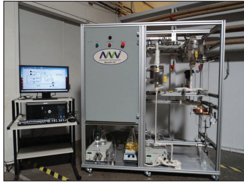
Figure 4. BenchCAT reactor for supercritical trans-esterification of lipids.
